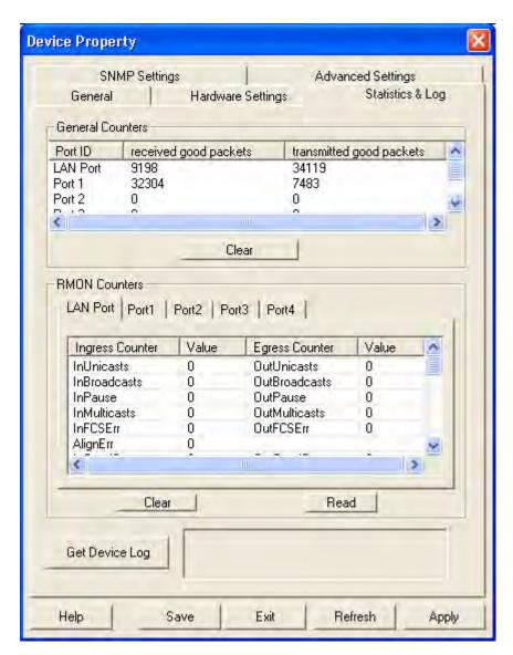
From this view you can see statistics about the number of good or bad packets each port has received and transmitted, based on how you have configured the Counter Mode setting (see step 7 on page 36).
